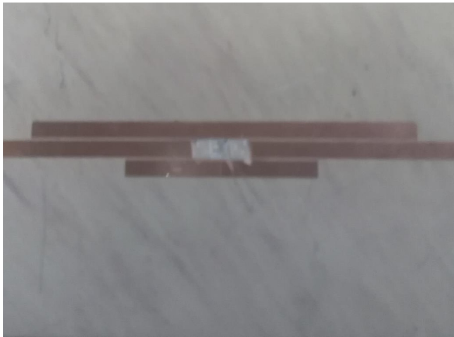
Fig. 1. Band-pass filter with "half-wave" and "wave" resonators connected in parallel
