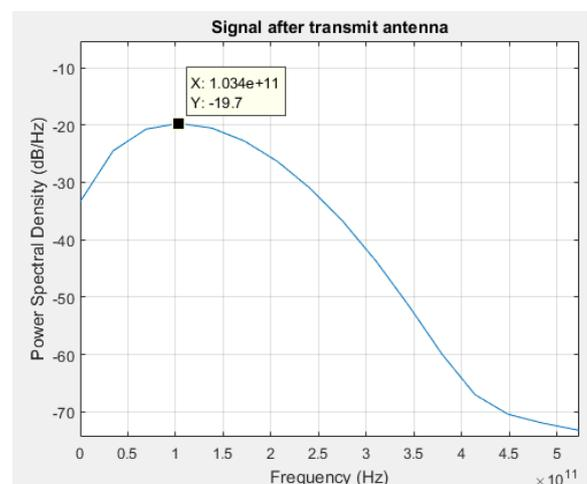
Fig.2. Spectral density of pulse in channel.
