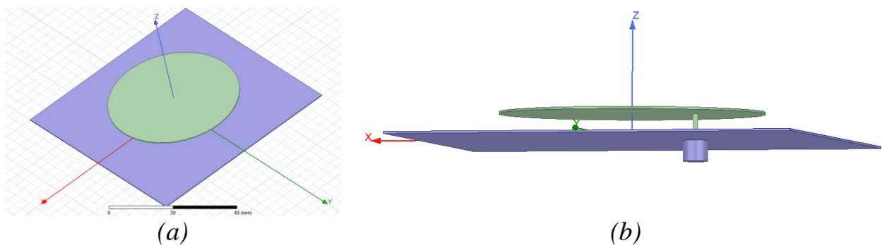
Fig.2. Model of the antenna. (a) Upper view. (b) Side view
