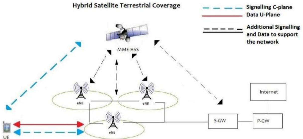
Fig. 1. Hybrid satellite terrestrial system architecture
