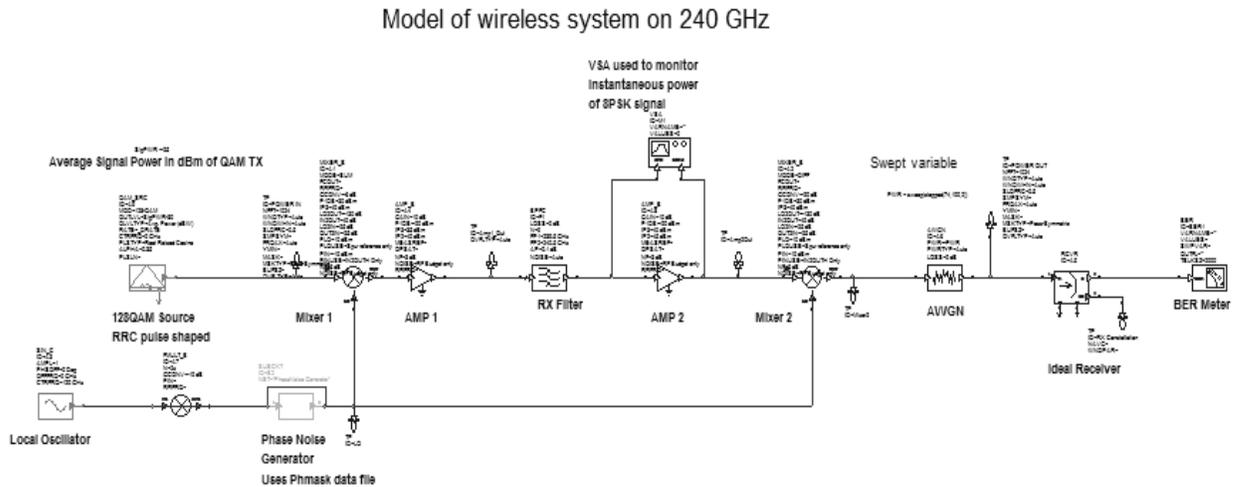
Fig. 1 The model wireless system
