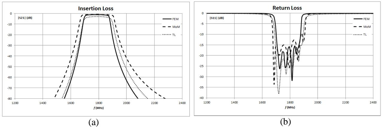
Fig.3. Frequency responses of the filter calculated by different numerical techniques.
